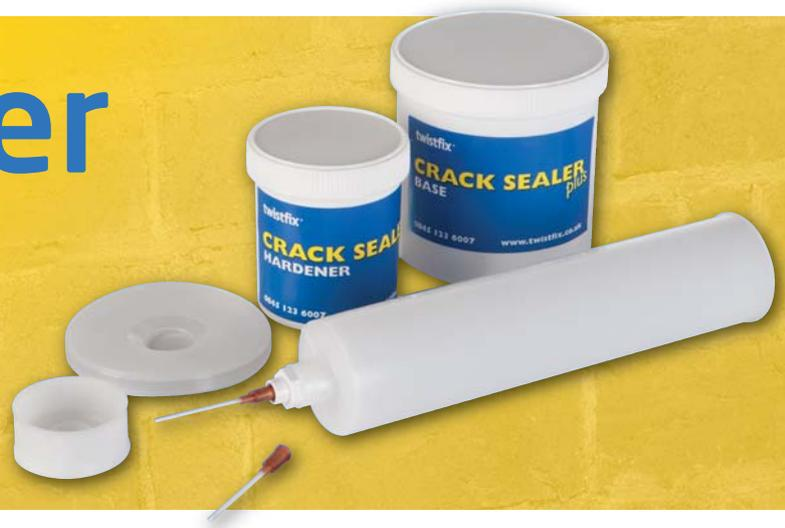
**Twistfix<sup>®</sup> Crack Sealer Plus** is a 2-part thixotropic epoxy adhesive. It may be used in film thicknesses between 0.2mm and 12mm. **Twistfix<sup>®</sup> Crack Sealer Plus** is specifically formulated for repairing fine cracks in brick, block, stone, concrete or masonry.
