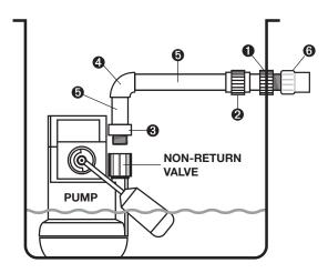
First select a suitable location for the pump ensuring that the float arm is not obstructed by for example the tank wall, inlets etc, at it's optimum reach. Remove the nut located in the pump switch and push the float arm into place ensuring that the nut is securely replaced. Prior to installing the internal pipework please check the Non-Return Valve is securely fixed to the pump outlet and ensure that the flap opens in the direction of the flow.
