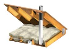
Cellulose insulation has its disadvantages. When improperly installed, there can be gaps around pipe penetrations as shown. Dryblown cellulose can settle, creating additional air pockets. It can also absorb moisture, significantly reducing its thermal value and allowing the potential for mold and mildew growth. FROTH-PAK™ products, when installed properly, expand to form an airtight seal – even around penetrations. FROTH-PAK™ foam does not settle and resists moisture penetration.
