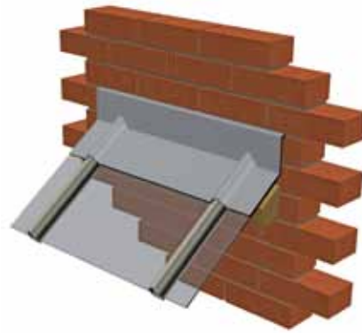
Figure 09: flashing to a top abutment - patent glazing
