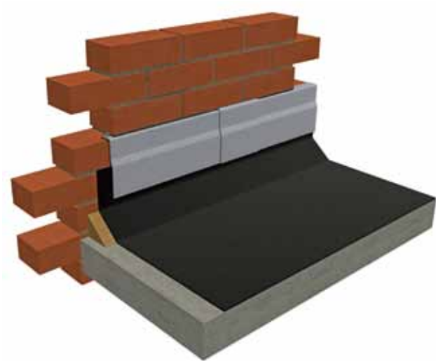
figure 04 Flashing to a flat roof upstand
