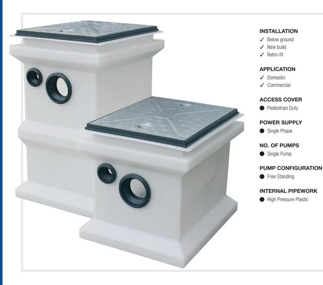
The MagnaStandard is a fully automatic small bore pumping station suitable for pumping foul, storm or surface water to a higher level when gravity drainage is not possible and/or economical to install.
