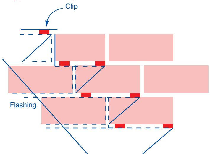
2. Completed installation of the clip into the standard brick joint
