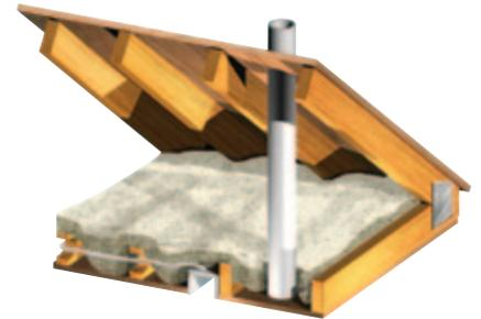
Cellulose insulation has its disadvantages. When improperly installed, there can be gaps around pipe penetrations as shown. Dry-blown cellulose can settle, creating additional air pockets. It can also absorb moisture, significantly reducing its thermal value and allowing the potential for mold and mildew growth. FROTH-PAK™ products, when installed properly, expand to form an airtight seal – even around penetrations. FROTH-PAK™ foam does not settle and resists moisture penetration.
