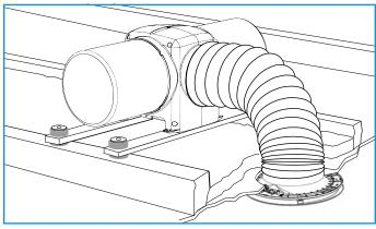
Place anti-vibration mounts above and below each batten fixing point and, using the 4 large screws and special washers, fix the unit to the joists. **Do not overtighten the fixings. The distance from the top washer to the joist when installed must not be less than 50mm.**
