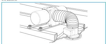
Place anti-vibration mounts above and below each batten fixing point and, using the 4 large screws and special washers, fix the unit to the joists.
